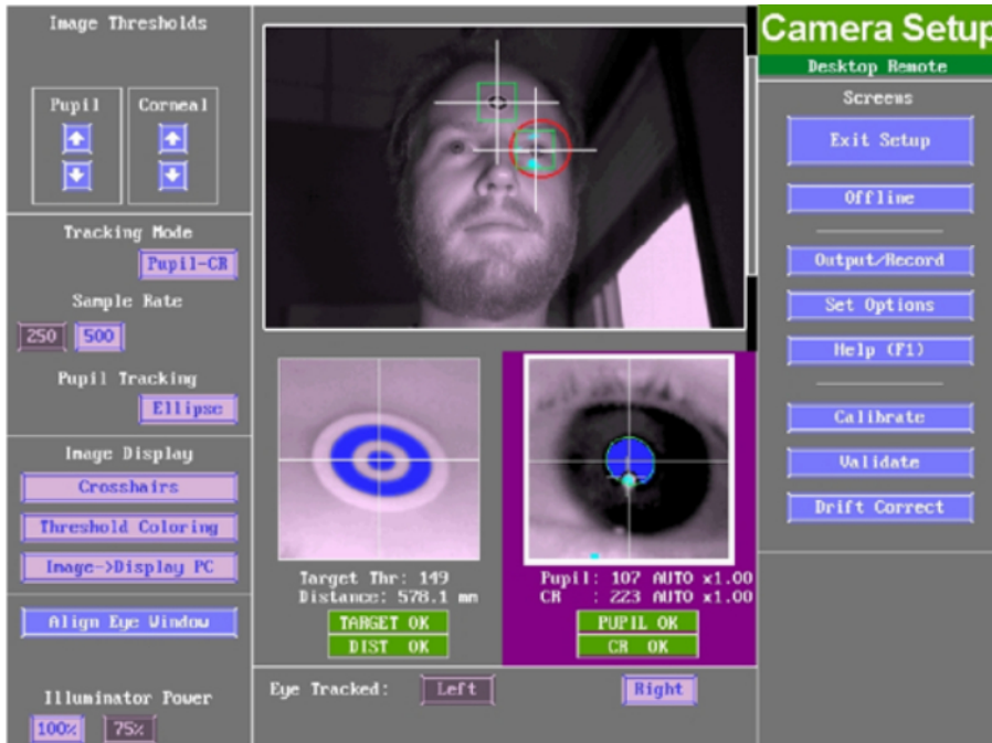
Figure 2. Example eye tracker camera setup screen. Target marker bounding box, eye bounding box, head distance, pupil, and corneal reflection (CR) should be marked as green and/or “OK” before proceeding. Please click here to view a larger version of this figure.
